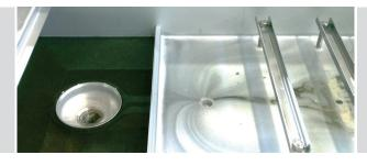
The RTG hydraulic unit extracts the floating oils and particles in the DPS 120 coalescence oil separator.
