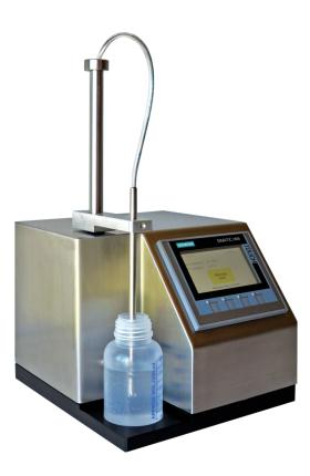
The RTG TENSIOTEST T90 determines the amount of the free surfactants in the cleaning agent by measuring the dynamic, volumetric surface tension. To achieve that, the T90 is calibrated with the surfactant that is used. After that, the current cleaning efficiency can be determined reliably and fast (display in %).
